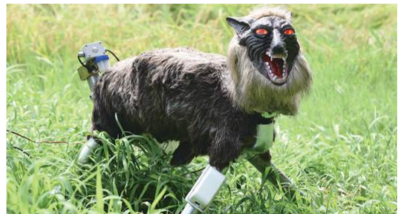
A wolf-like robot “Super Monster Wolf” stands beside a rice field to drive away wild animals that cause damage to crops in Kisarazu, Chiba prefecture, Japan, on August 25, 2017. – AFP
