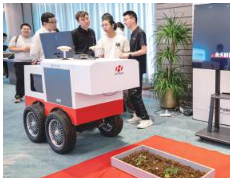
Visitors learn about the Hg LaserWeeder, a 24/7 intelligent laser weeding robot at a product launch event in Wuhan, capital of Hubei Province, on Saturday. A laser weeding robot is an advanced agricultural machine that uses laser technology to eliminate weeds without chemicals or manual labor. These robots are part of precision farming, helping reduce herbicide use, lower environmental impact, and improve crop yields. – Xinhua/DeepSeek
